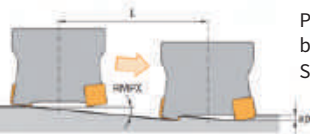
Figure Illustration of ramp milling
